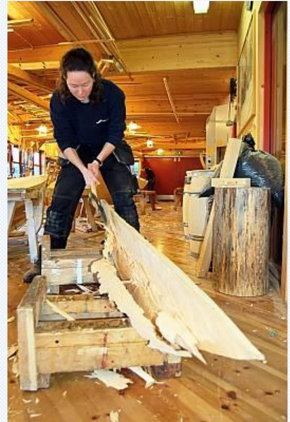
Boat-builder Berit Osmundsen shaping a garboard, a plank in the bottom of an Oselvar boat© Kjell Magnus Økland, 2015
